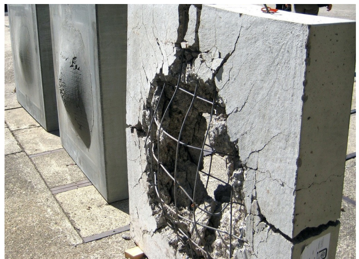
Rear: DUCON vs. reinforced concrete (right)
