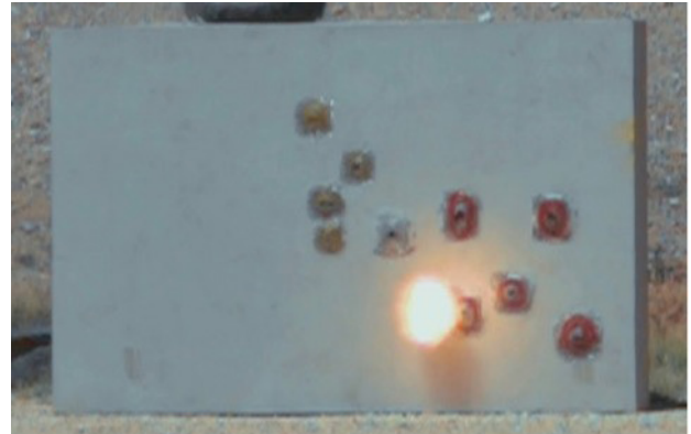
Picture: Firing tests with 12.7mm x 112mm hard core bullet incl. incendiary composition (API)
