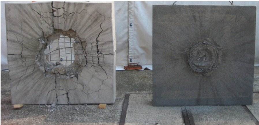
Fig. 24: Contact charge explosion test (Reinforced concrete on left, DUCON® on right), front
