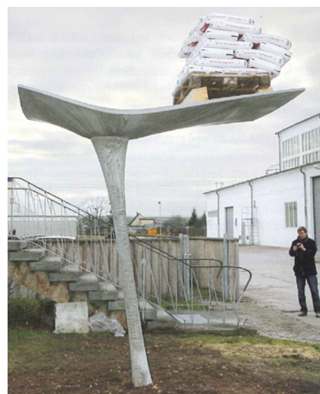
Fig. 6: Load bearing test on cantilever panel, 850 kg (1880 lbs)
