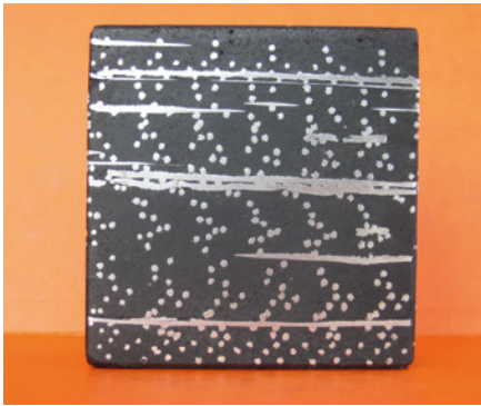
Fig. 1: Cross section of DUCON® (one variant), homogeneous distribution of micro-reinforcement
