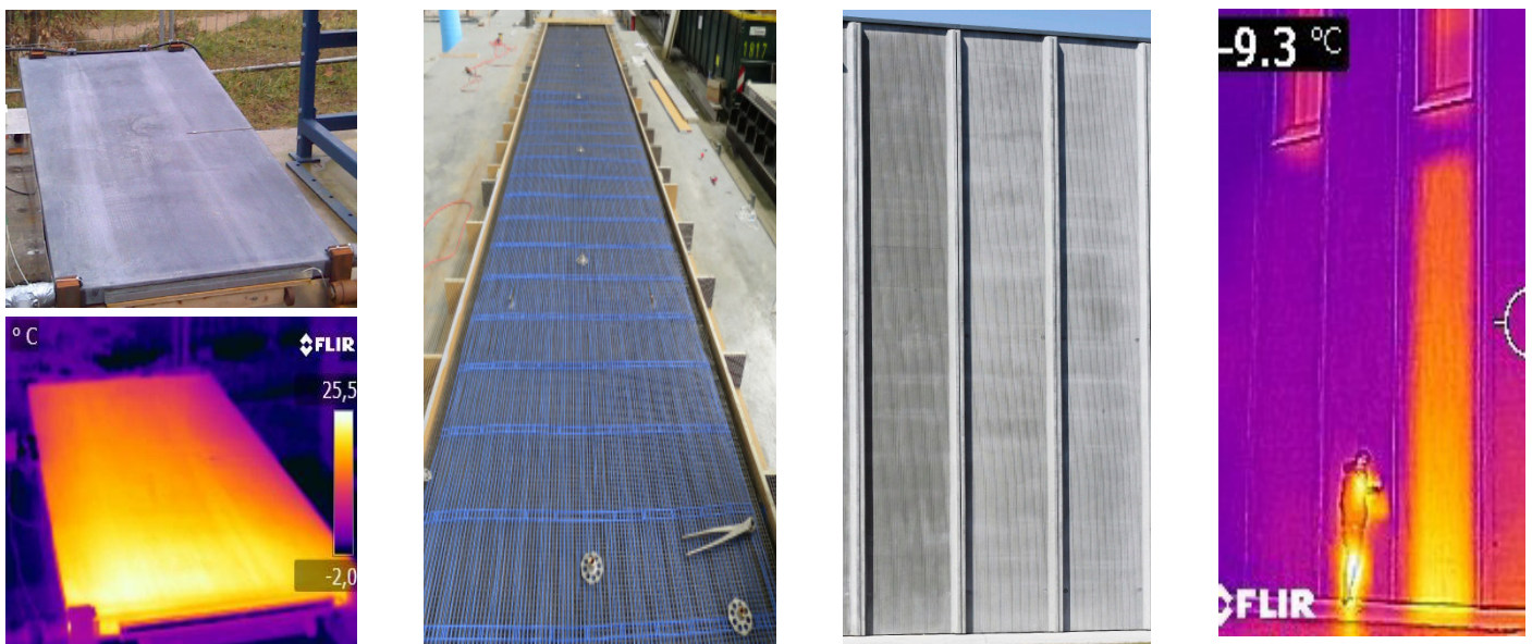
Figure: Production of thermally activated plate strips for heat recovery (glycol mixture)
